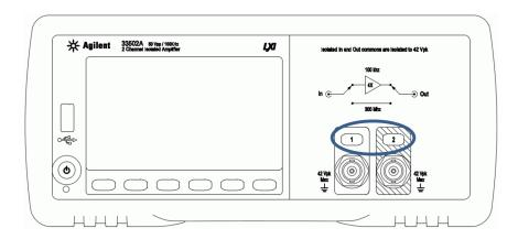
When you turn a channel on, the number on the button illuminates, as shown below for channel 1.
