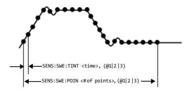
Figure 2-12 Commands that control measurement time
