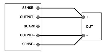
Figure 2-10 Remote sense connection
