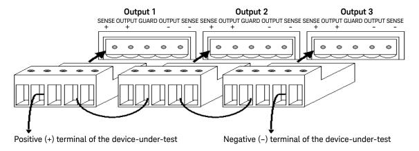
Figure 2-13 U2722A/U2723A outputs connected in series
