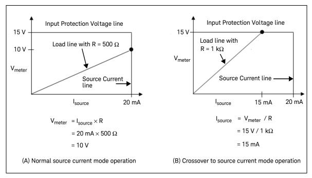
Figure 2-8 Source current operation
