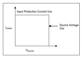
Figure 2-5 Source voltage positive operating boundaries
