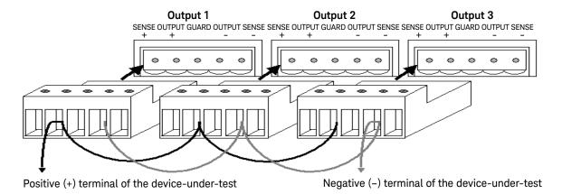
Figure 2-14 U2722A/U2723A outputs connected in parallel
