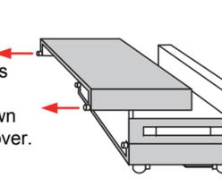
2. Install the power modules in the instrument.
