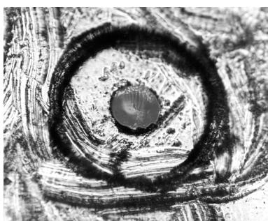
Figure 30 Damage from improper cleaning.
