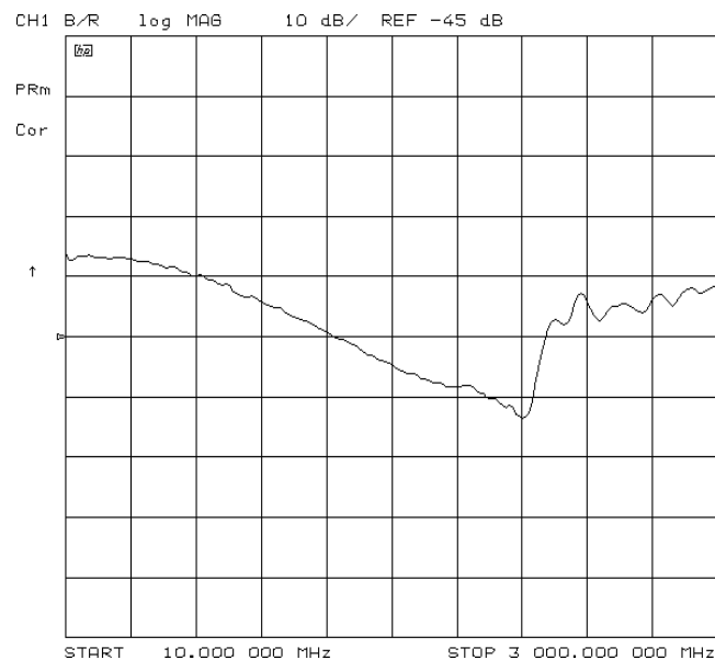
Figure 2-35 Example Mixer LO to RF Isolation Measurement
