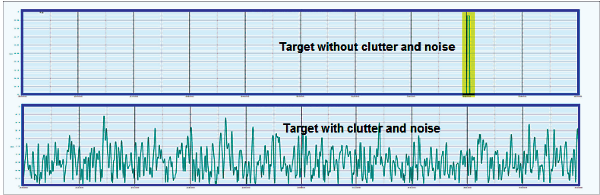
Figure 4.5. Target signal hidden by heavily cluttered environment
