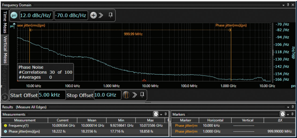
Figure 11.6. Infiniium Real-Time Oscilloscope phase noise interface.
