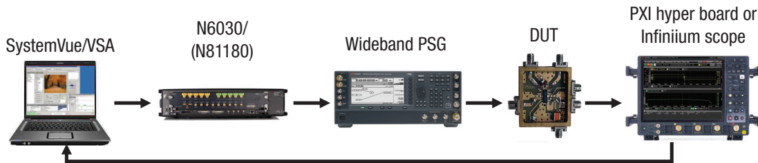
Figure 7.10. Test setup for wideband signal generation.
