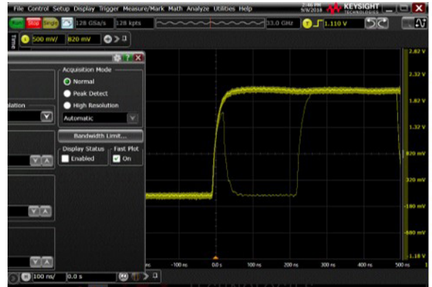
Figure 1. Fast plot, a hardware acceleration option, captured an elusive glitch on the UXR in just five seconds
