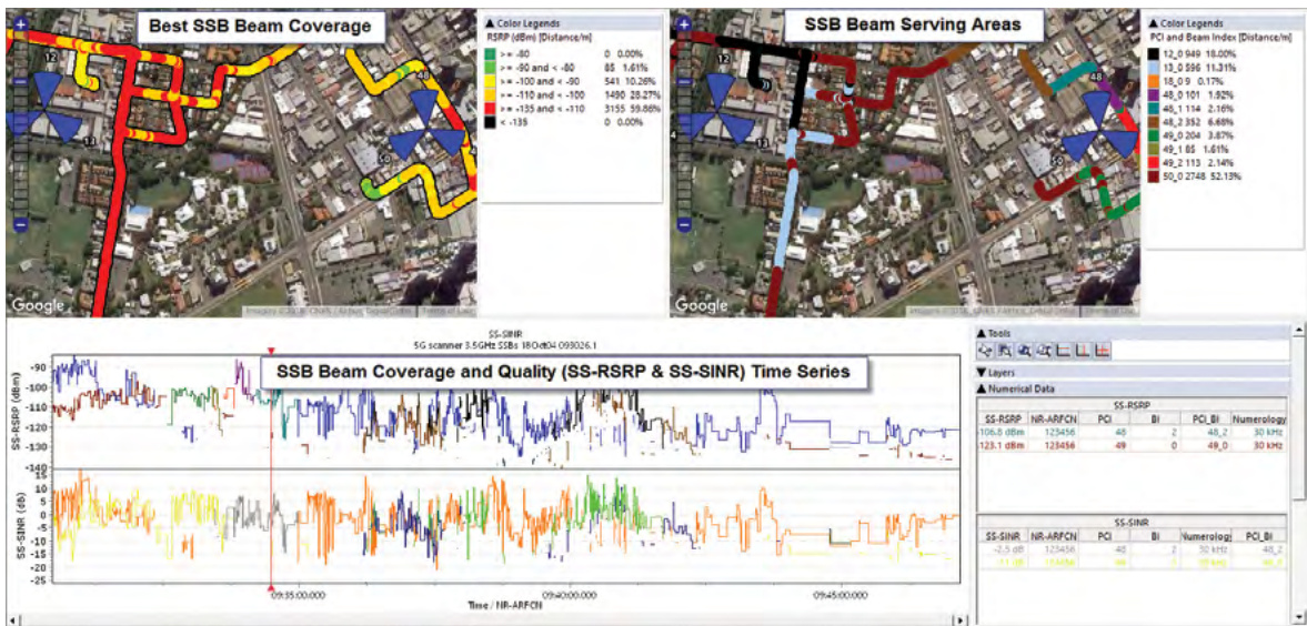
Figure 24.3. Example 5G NR scanner measurements showing coverage and quality metrics including SS-RSRP, SS-SINR per each SSB reference beam of a cell
