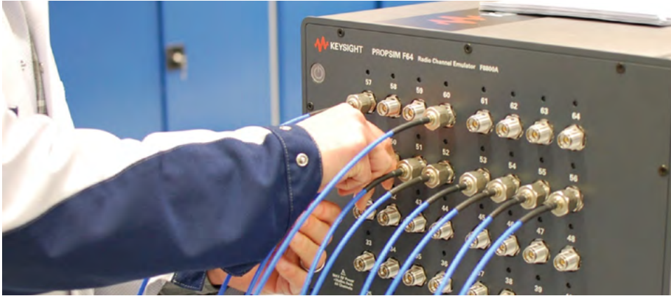
Figure 16.10. Ensure connectors are firmly attached and always use good quality cables
