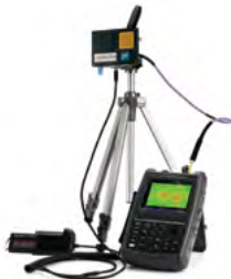
Figure 25.8. FieldFox phased array antenna coverage test system
