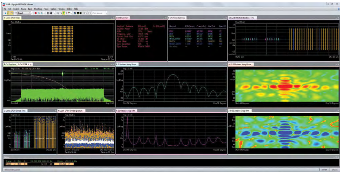
Figure 3.3. Analysis of a 5G NR 256 QAM signal with antenna pattern
