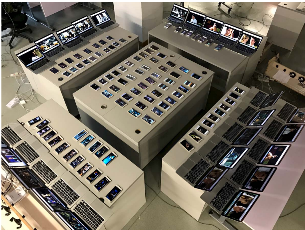
AP4030TN: High-Density Video Streaming Test Environment 120 Clients Streaming One HD Video Very Smoothly through One Huawei AP4030TN Access Point
