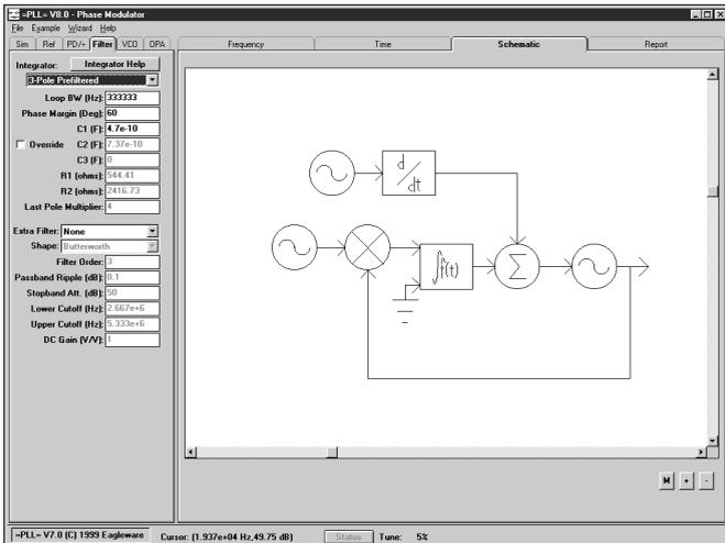
Schematic of a PLL used as a phase modulator.
