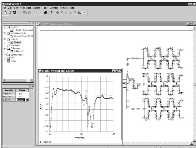
*This 400 element power splitter simulates 101 points in less than 2 seconds, tunes 101 points in less than 1/4 second on a 366 K6 PC.*
