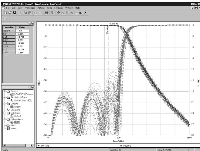
A sample Monte Carlo analysis of a lowpass filter, simulating 50 samples using a Gaussian distribution and tolerances of 5%.
