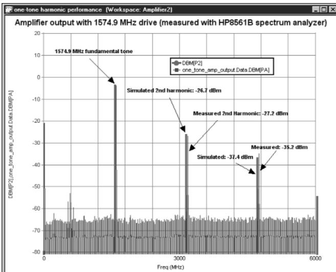
Measured and simulated single tone excitation of a 1.5 GHz GPS LNA. The measurement data was acquired with TEST LINK.
