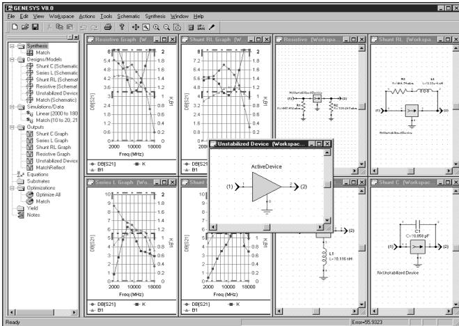
*GENESYS automatically designs a variety of stabilization networks. The user then chooses the most suitable solution.*
