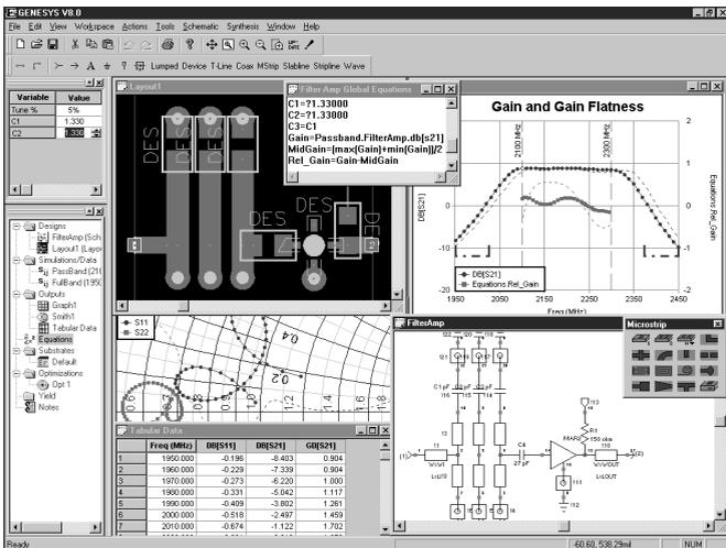
*Synthesis, schematic capture, circuit simulation, layout, and electromagnetic simulation are all integrated in the GENESYS environment.*
