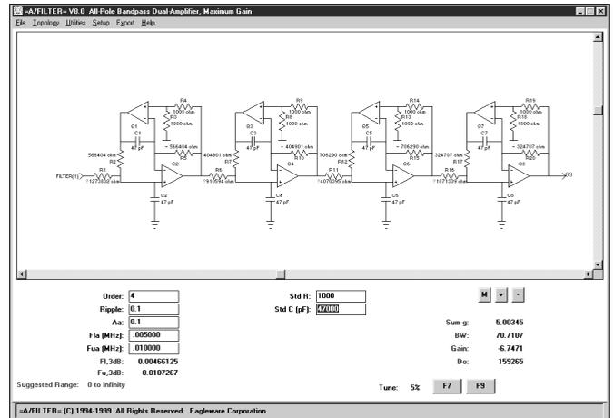
Synthesizing a Maximum Gain Dual Amplifier Bandpass Filter in A/FILTER.
