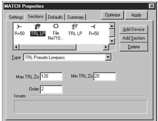
Setting up initial network parameters for a multistage amplifier.
