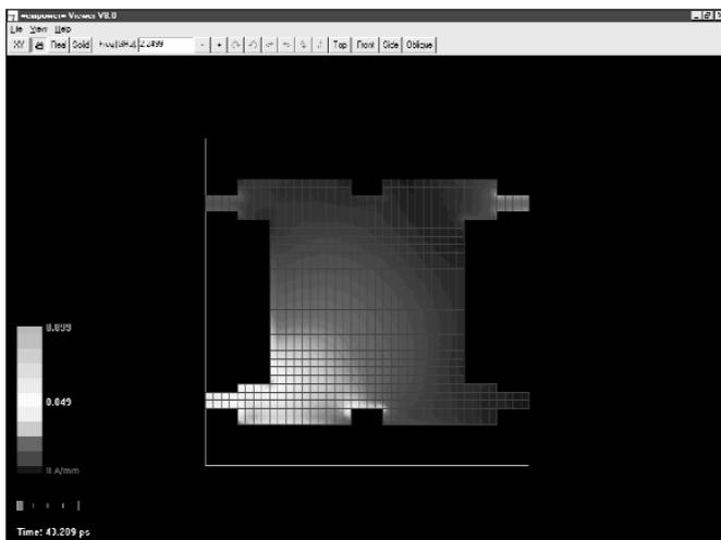
*A dualmode coupler in the EMPOWER viewer. An oblique view and a top view of the XY current magnitude. The port on the lower left is driven.*
