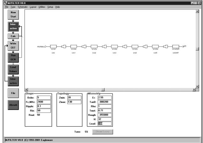
*Synthesizing a Stepped-z lowpass filter in M/FILTER.*
