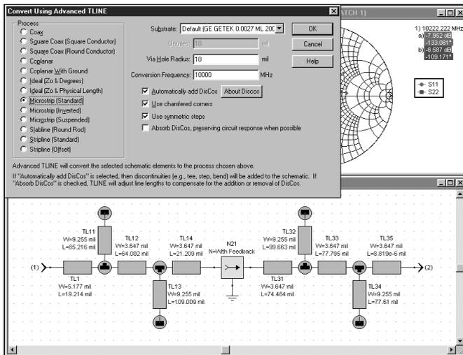
Advanced T/LINE setup dialog and matching circuit converted to microstrip.
