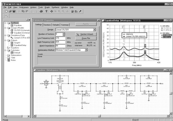
Five section group delay equalization of a 300 MHz bandpass filter.
