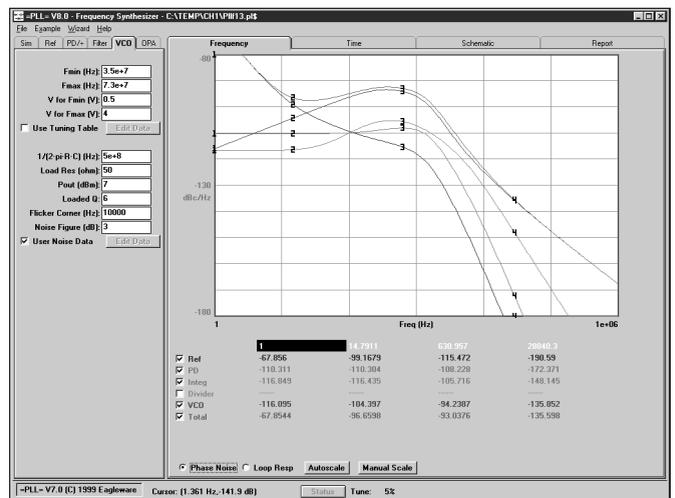
A PLL single side-band noise output window with a sweep from 1 Hz to 1 MHz carrier offset. The top trace is the total SSB noise at the output of the PLL. The remaining traces are the contributions to this total noise from the various loop components. These curves consider the action of the PLL on the original spectral noise plots of the offending components.
