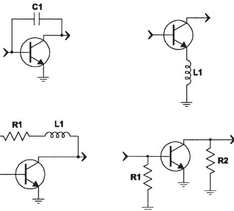
*Devices are stabilized by applying any of the built-in templates to optimize feedback element(s) for unconditional stability conditions.*
