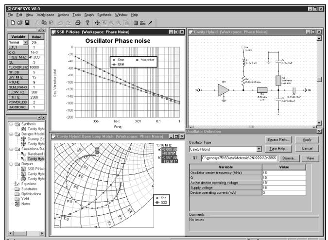
GENESYS screen showing SSB phase noise analysis of the cavity hybrid VCO.
