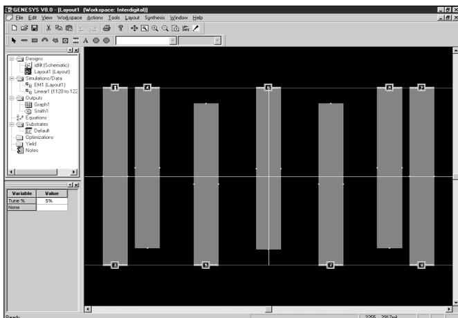
*The layout of an interdigital filter. You can export a DXF or Gerber file that is sent to the PCB/PWB manufacturer or you can use with your own PWB milling machine.*
