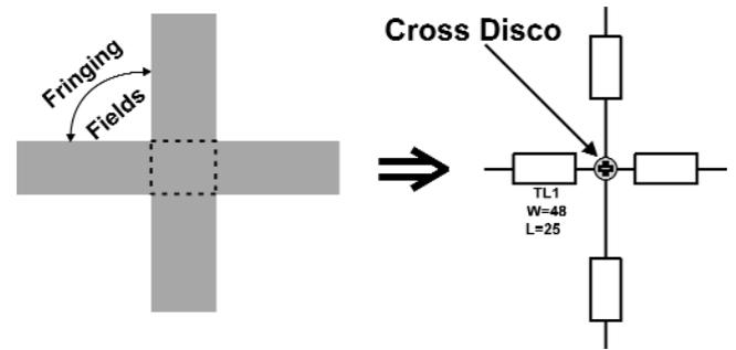
Physical and schematic representation of two crossed microstrip lines. Fringing fields exist at all four corners of the intersection, and are only modeled when using discontinuity models. Advanced T/LINE automatically inserts these models as needed.
