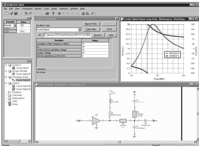
GENESYS screen showing OSCILLATOR synthesis of a cavity hybrid VCO.
