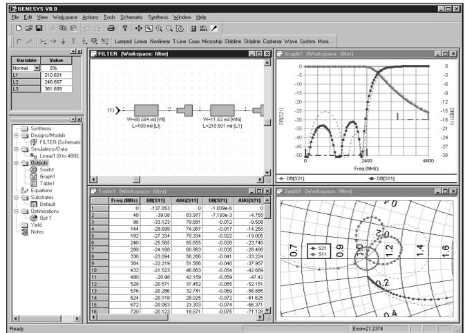
*M/FILTER design being tuned and optimized in GENESYS.*
