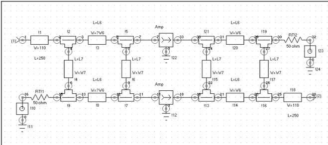
Schematic of a Balanced Amplifier.
