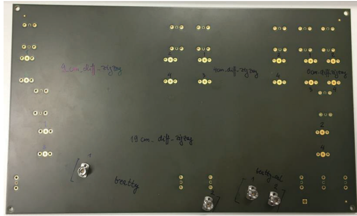
Figure 13: Stripline Beatty standard example test PCB.
