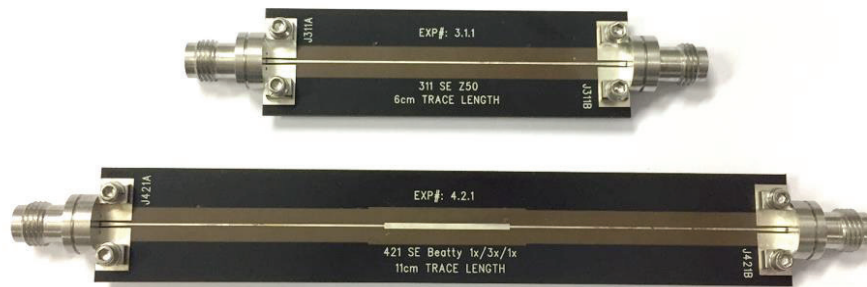
Figure 21: Single-ended microstrip Beatty standard example.
