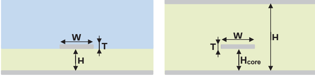
Figure 4: Cross-section of microstrip (left) and stripline (right).
