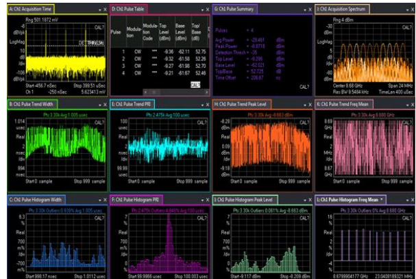
Figure 2. Automatic Pulse Analysis with Keysight 89600 VSA
