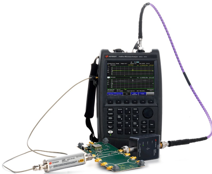
Figure 1-2. Keysight FieldFox handheld microwave analyzers with noise figure measurements
