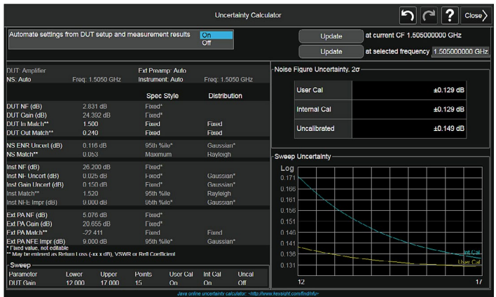
Figure 5-2. X-Series NFA noise figure analyzers and X-Series signal analyzers with noise figure measurement application have a built-in uncertainty calculator with graphical results that can auto-populate instrument, preamplifier and noise source parameters.
