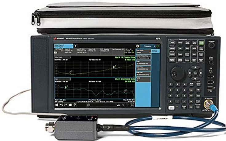
Figure 6-3. If the instrument noise figure is high, a low noise preamplifier will reduce the effective instrument noise figure. If the preamplifier is external, ensure it is included in the calibration loop.
