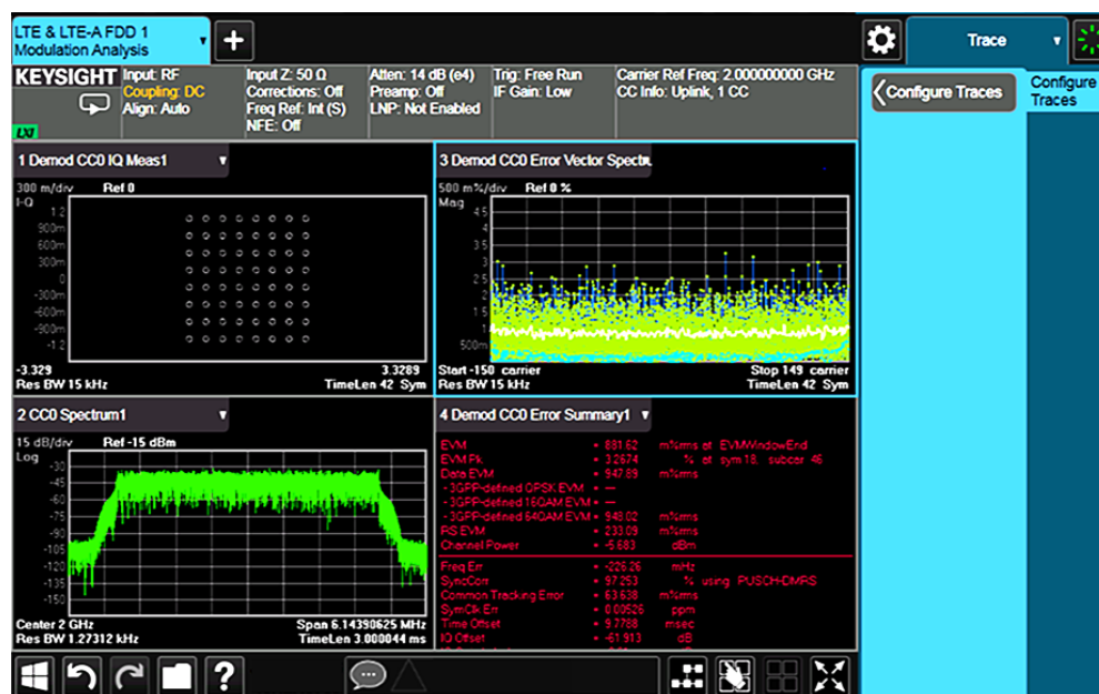
Figure 8-6. EVM measurement of LTE FDD downlink signal
