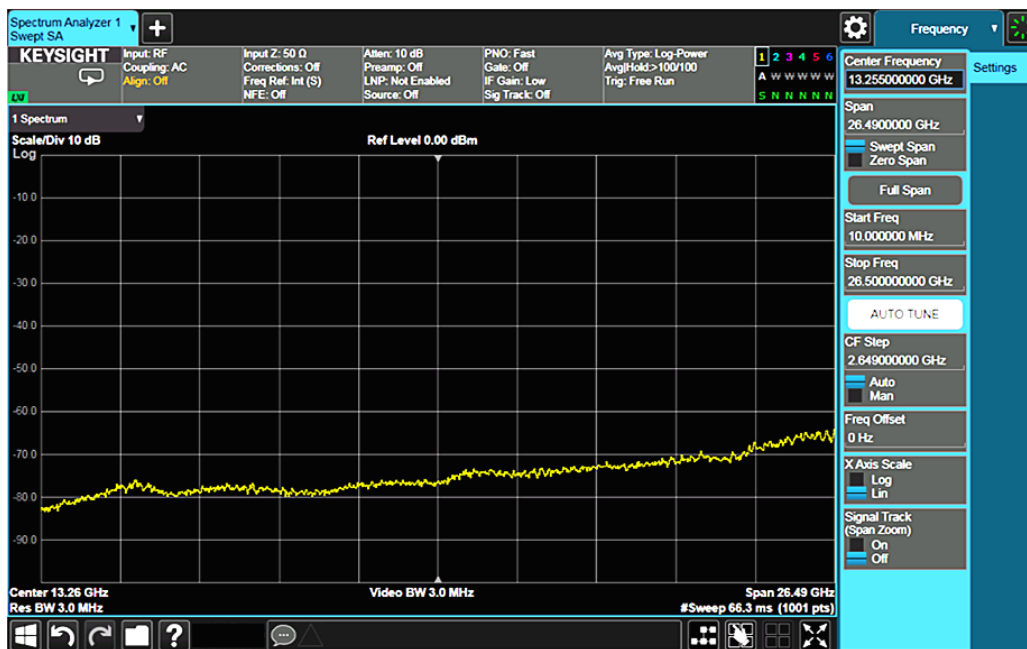
Figure 7-10. Rise in noise floor indicates changes in sensitivity with changes in LO harmonic used
