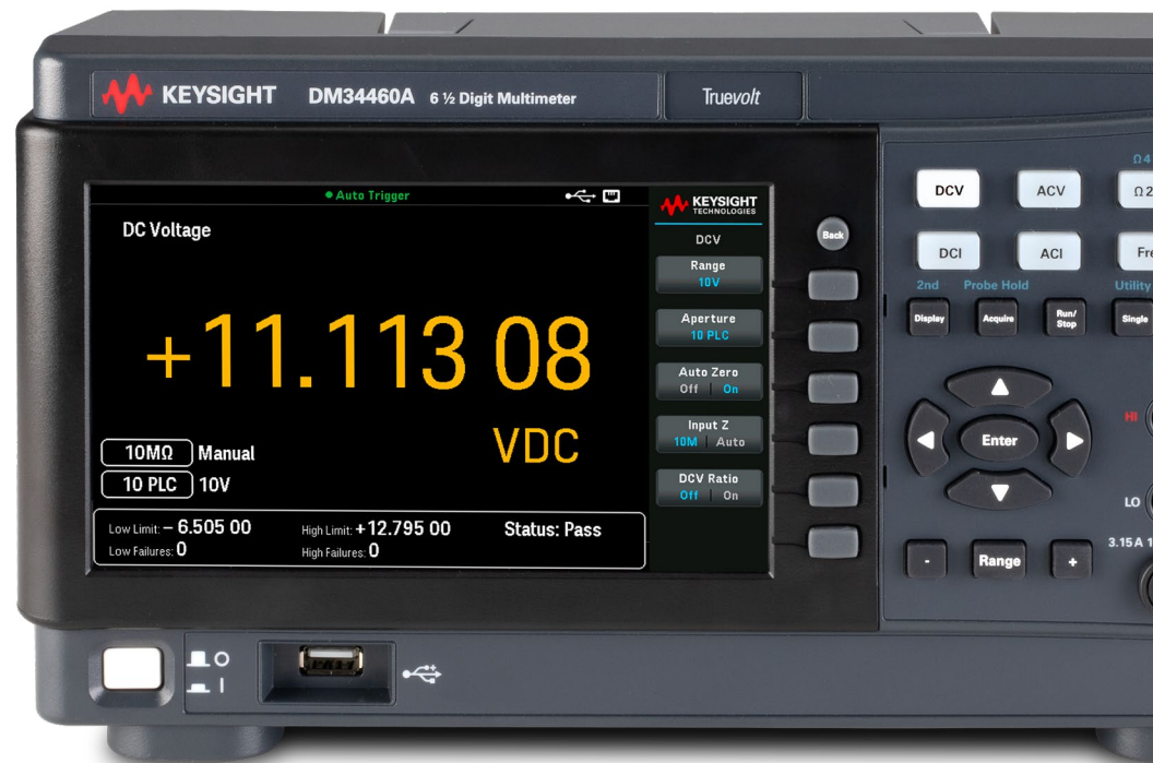
Figure 1. Keysight benchtop digital multimeter displaying 6.5 digits of resolution
