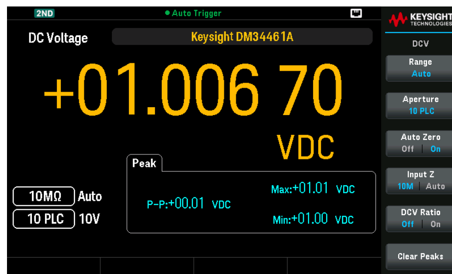
Figure 3. Smart Bench Essentials Plus DMM with a large 7-inch dual display
