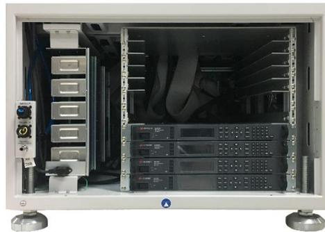
Figure 1: System bottom, 10 RU space for additional hardware
