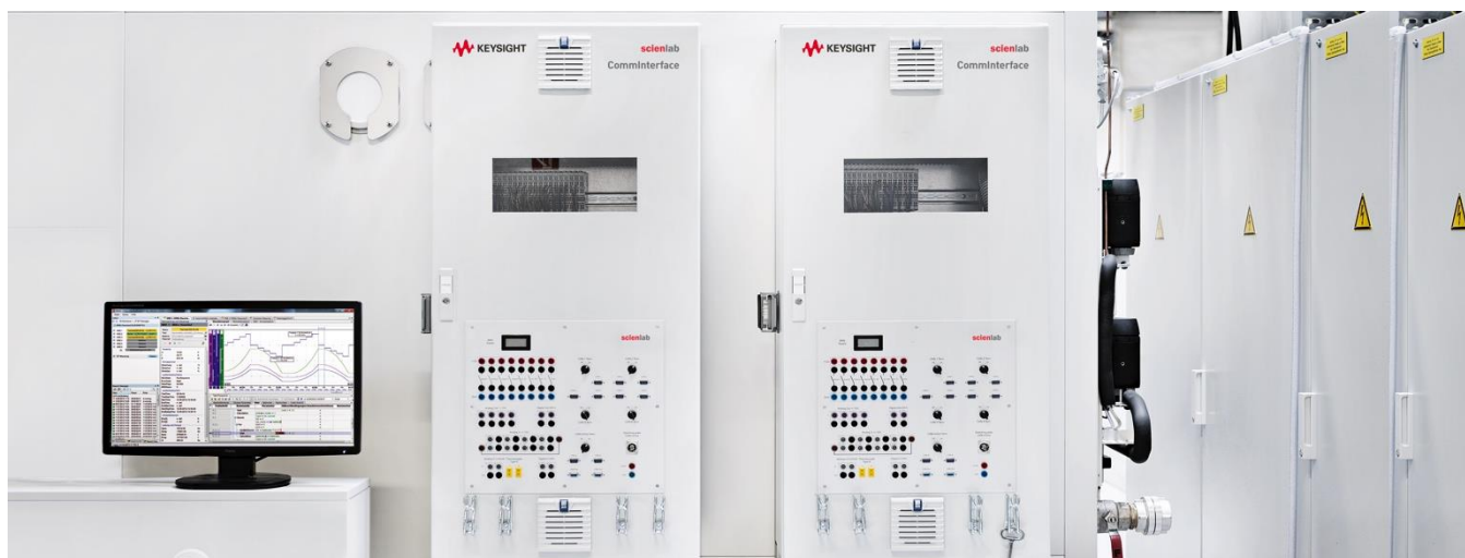
Test bench controls with communication interface connected to the DUT (CommInterface)
