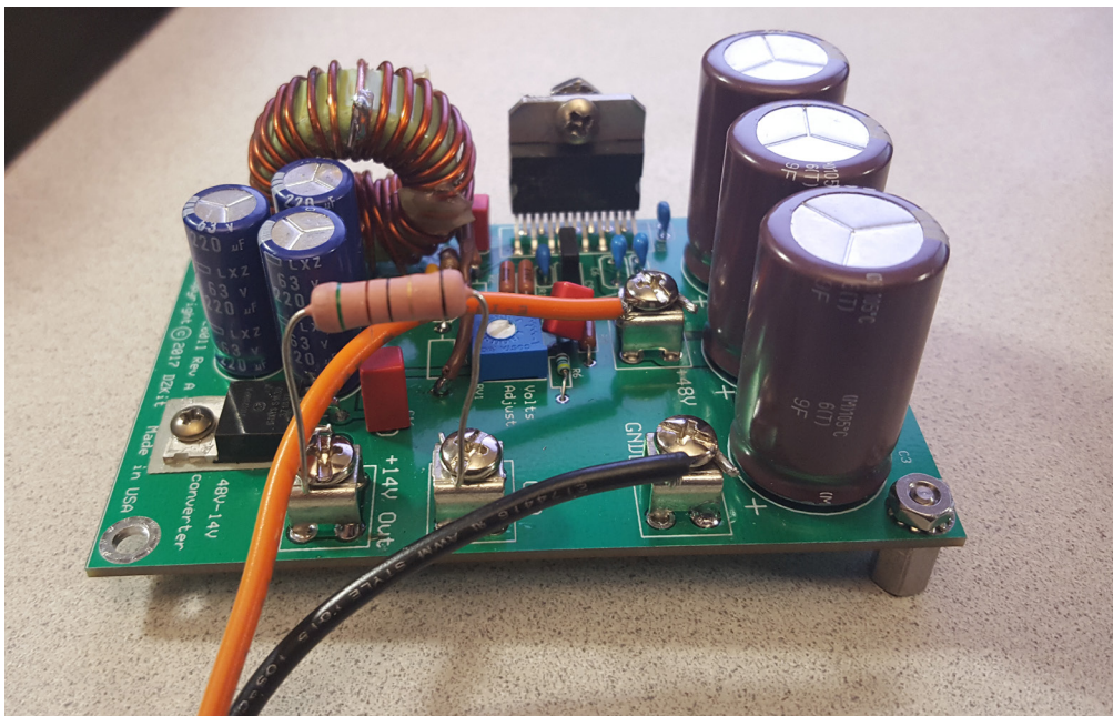
Figure 1. DC-DC converter using ST Technologies L4975A IC.
