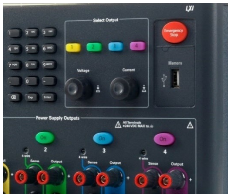
Figure 11. The N6705's front panel USB port.
