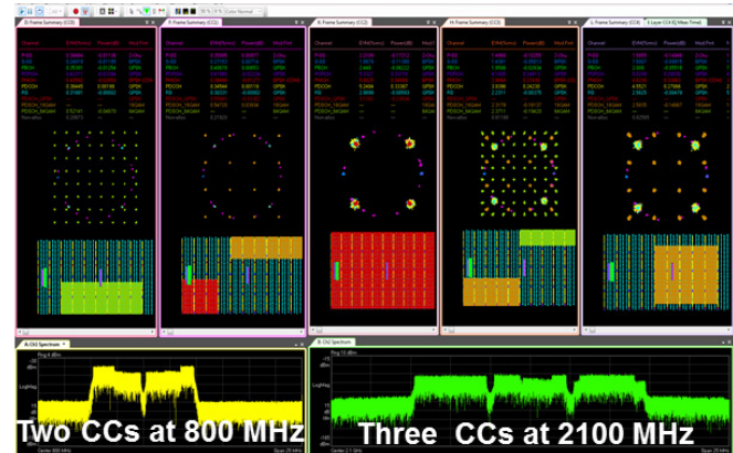
Figure 2. 89600 VSA software for inter-band carrier aggregation analysis.
