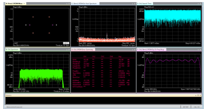
Figure 8. The M9703A wideband digital receiver allows to directly digitize DVB-T signals with excellent dynamic range without the need of analog mixers, especially interesting for passive radar applications.
