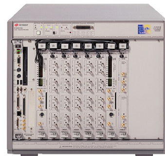
81250 modular BERT platform (used for the E4887A, TMDs Generator)
