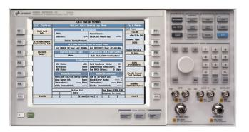
RAT tests such as connected data handover, SRVCC, CSFB, and RRC release with redirection.
