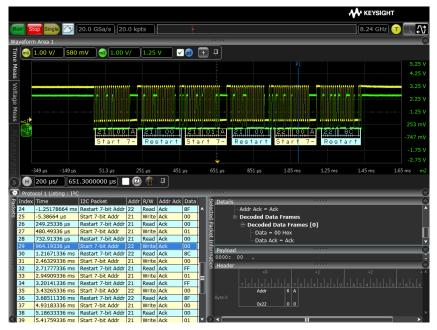
Quickly move between physical and I2C protocol layer information using the time-correlated tracing marker. Display protocol content using embedded decode in the waveform area, Or, see protocol events in a compact listing format using the industry's first scope based multi-tab protocol viewer. For I2C minor tick marks indicate clock transitions. Major tick marks indicate sections of the serial packet such as address, acknowledge, and data.
