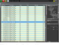
Fill the entire display with compact protocol information. The protocol viewer shows index number, time stamp, and data content for each serial packet. Listing content can be saved to a .csv or .txt file for off-line analysis or documentation. Use search capability to quick navigate through an acquisition.
