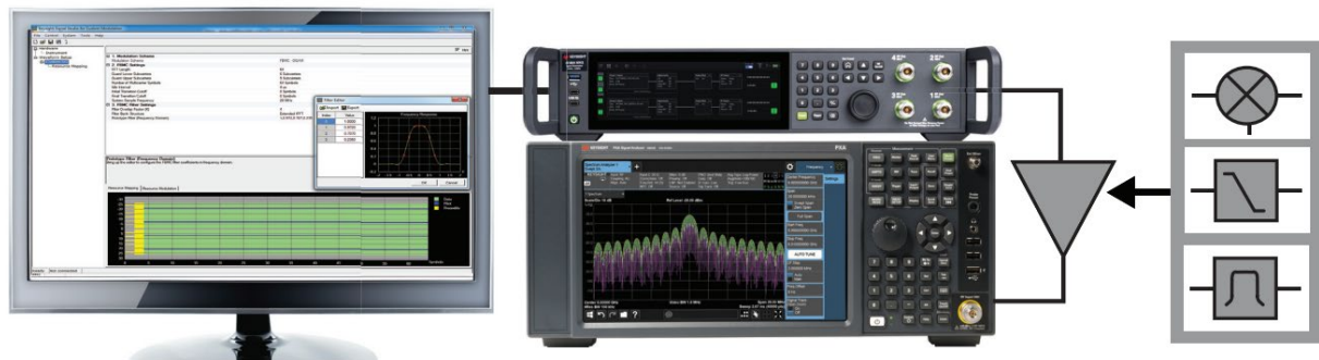
Figure 2. A typical component test configuration using Signal Studio with Keysight signal generator and analyzer
