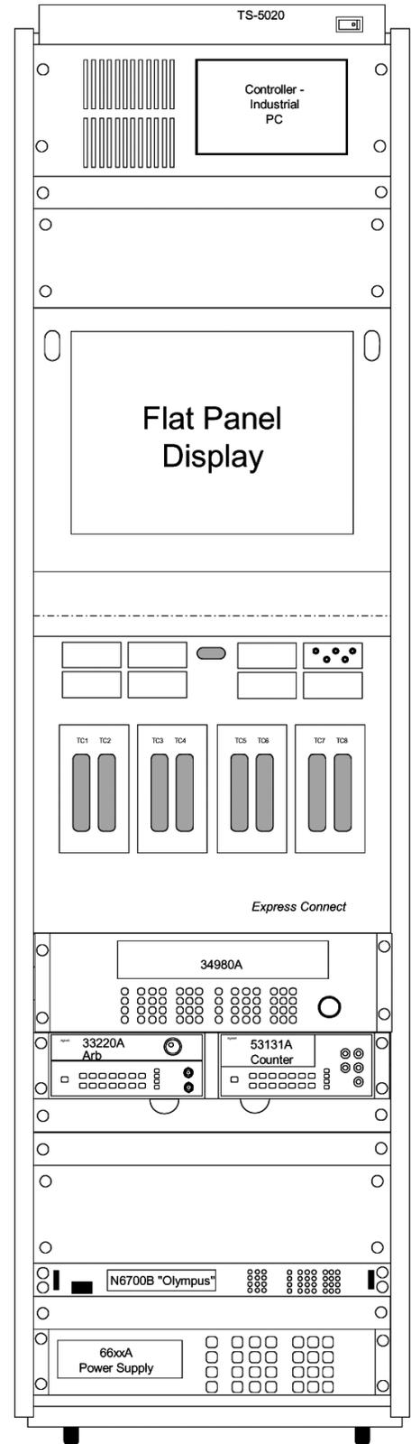
Figure 2. Keysight TS-5020 automotive functional test system
