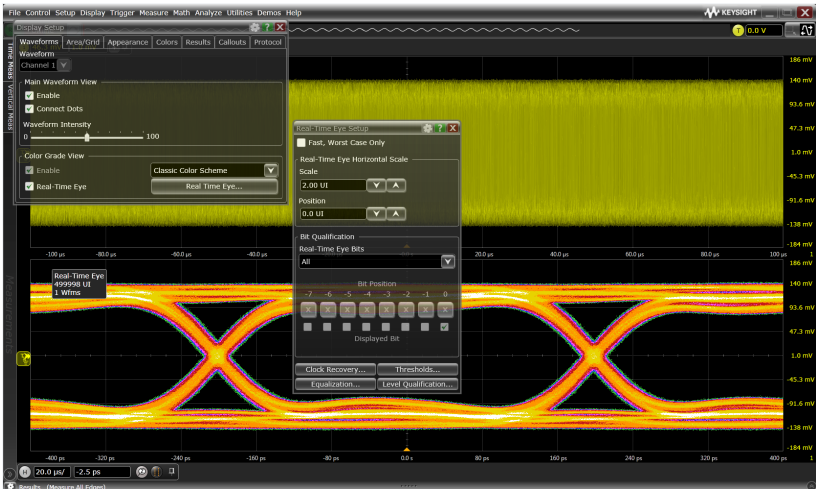
Figure 6. To set up a measurement, the wizard asks you to identify the signal source and select the clock recovery algorithm.
