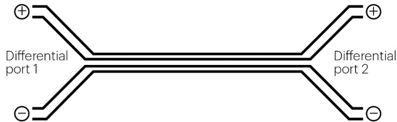
Figure 18. Differential S-parameter model
