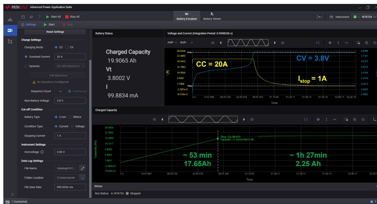
Figure 11. Capacity stored in the battery while charging a fully discharged battery in constant current mode with a current of 1C = 20A , from 2.4V to 3.8V , and then CV mode with a current stopping limit of 0.05C = 1A . Stored capacity 19.9 Ah.
