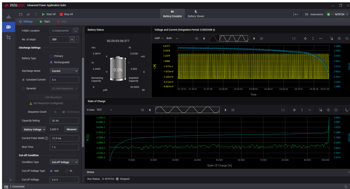
Figure 9. Battery modeling test with discharge current of 0.2C = 4A, current pulse width 12.5 ms, rest time = 1s and cut-off voltage Voc = 2.4 V
