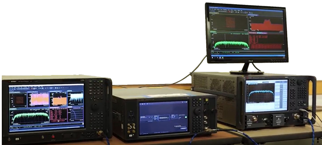
Figure 2. DVB-S2/S2X measurement system
