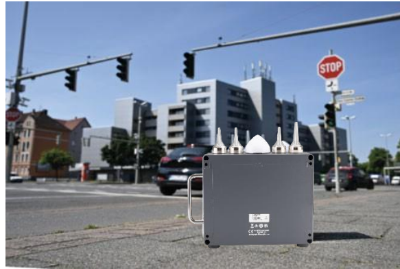
Figure 3. WaveBee Togo simulating vehicles for RSU testing at intersection
