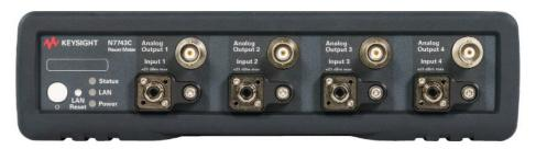
For measuring optical power levels above +10 dBm, the N7743C is a good fit to devices like transmitter lasers, with +20 dBm maximum input power. The dark noise level is less than 30 pW, providing over 90 dB dynamic range. This provides an intermediate performance alternative to the remote heads, like the 81626C or 81628C that cover still higher power levels.
