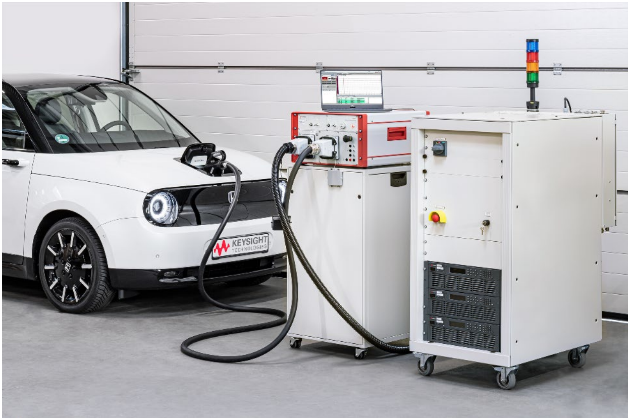
SL1202A 45 kVA AC Emulator with SL1040A Charging Discovery System for EV and EVSE charging test
