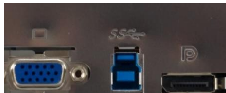
Presence of USB 3.0 and DisplayPort: CPU/motherboard can run Windows 10
