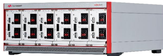
SL1004A Tabletop device (12 channels 5 A)
