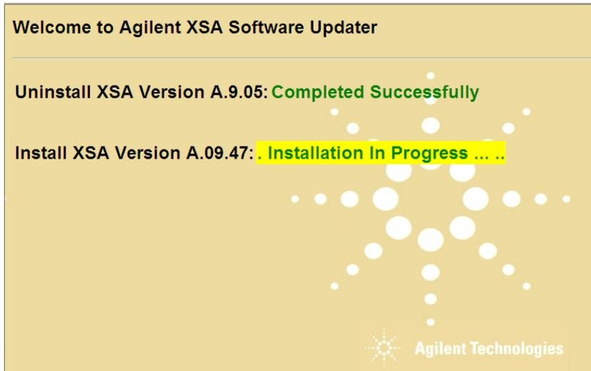
The new instrument software is being installed. The “Installation in Progress” text will roll across the screen indicating software activity. There will be several windows appearing and disappearing during this time. NO interaction with the instrument is required. Please be patient the total software installation process can take 35 to 40 minutes. It will display “Completed Successfully” when the software update is complete. You will be prompted to restart your instrument at the end.
