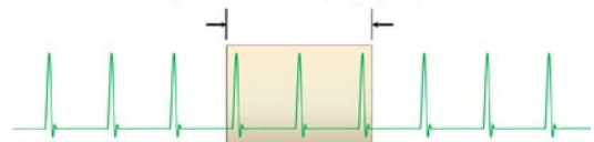
Figure 1: Continuous acquisition time is a function of a scope's memory depth and sample rate.
