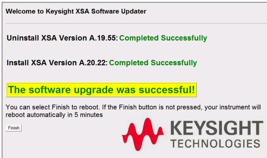
4. When the Software installation is complete. You will be asked to reboot the instrument. If no action is taken the instrument will automatically reboot in 5 minutes.
