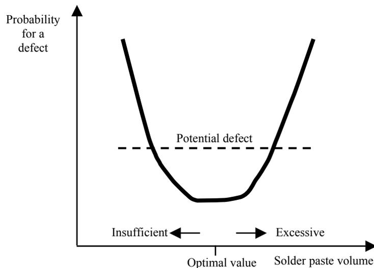
**Figure 3. The concept that a potential defect(s) may or may not be defects at the end of the manufacturing process.**
