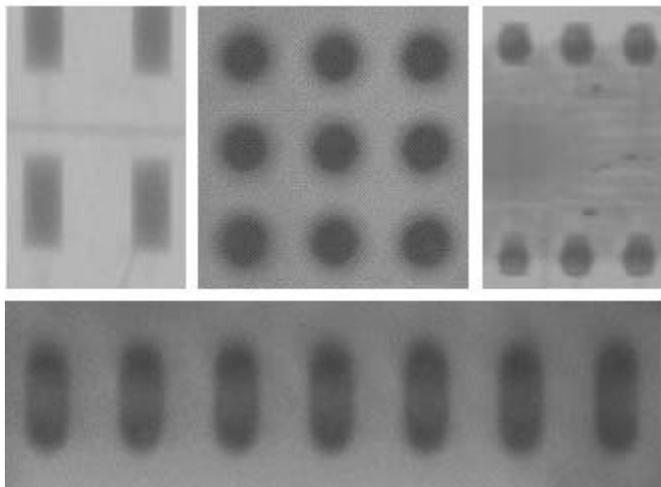
Figure 5. X-ray images of lead-free solder.
