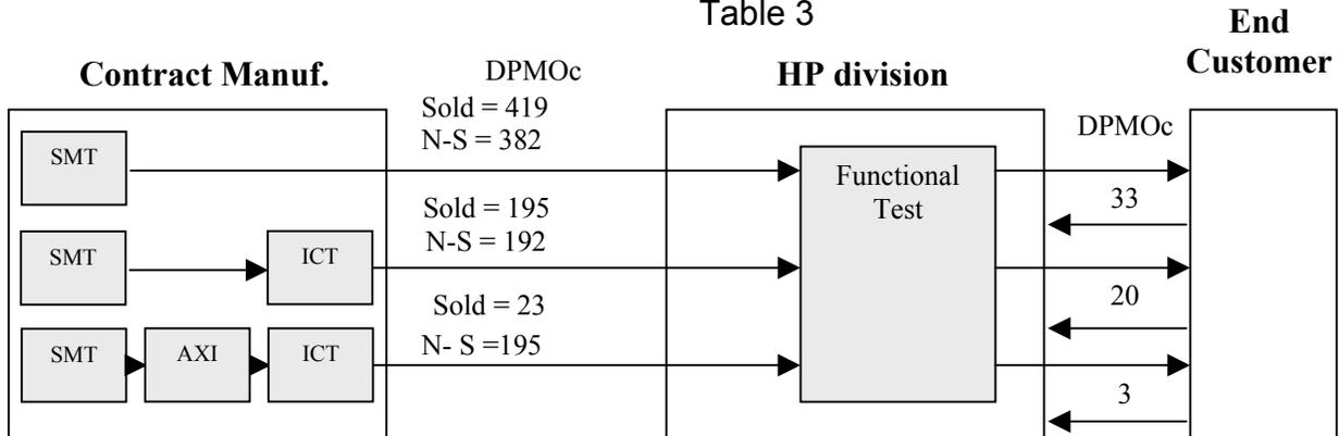
Total of 6,928 boards in the study. Sold = Solder defects. N- S = Non solder defects.
