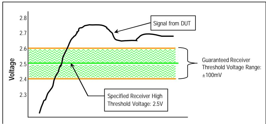
Figure 3 Receiver high threshold range
