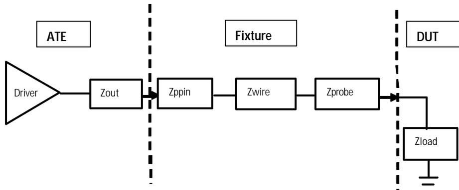
**Figure 5 Impedances during digital testing**
