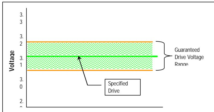
Figure 2 Driver voltage range ( $\pm 100\text{mV}$  accuracy)
