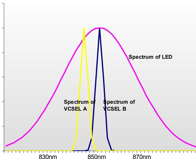
Fig 2: The spectrum of a VCSEL is narrow and different devices may have slight offset in the central wavelength. The spectrum of an LED, on the other hand, is much broader.
