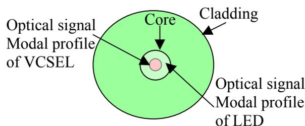
Fig 1: The optical signal from LED covers larger part of the fiber cross-section during the test, uncovering fiber formation defects
