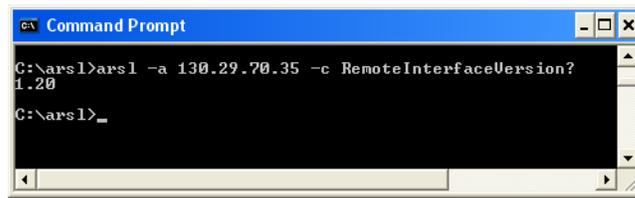
In the example, the utility is running on a PC, the automated test application is running on an oscilloscope at IP address 130.29.70.35, and the command being sent is a property query to discover the version of the app's remote interface (1.20).
