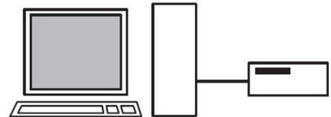
\*Directly connecting an instrument to a PC with LAN may require a special LAN Crossover Cable.
