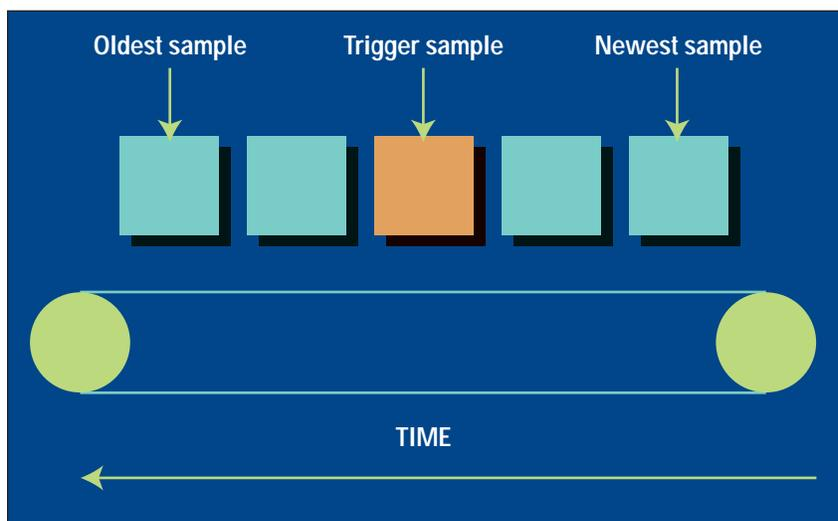
**Figure 1.** A logic analyzer is analogous to a conveyor belt. As new data enters, old data falls off the end.
