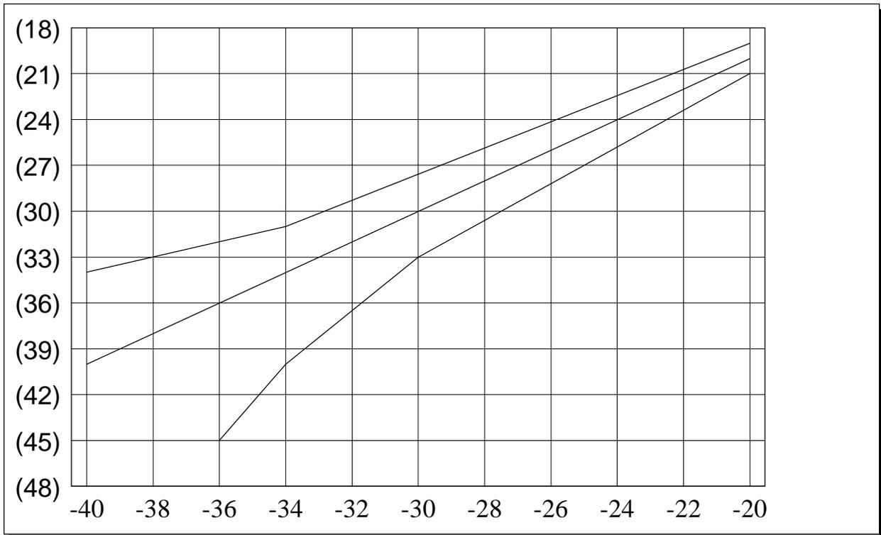
**Figure 5. Return Loss of Device-Under-Test**
