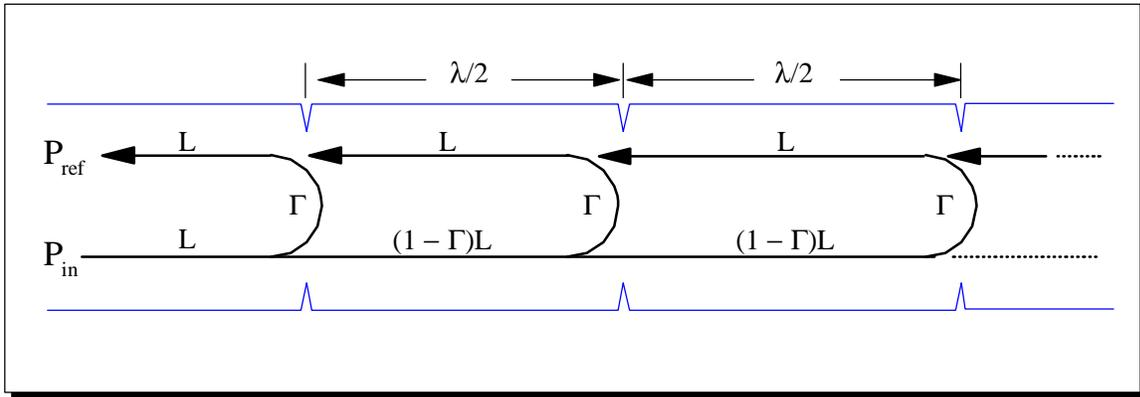
**Figure 1. Periodic bumps in a cable**
