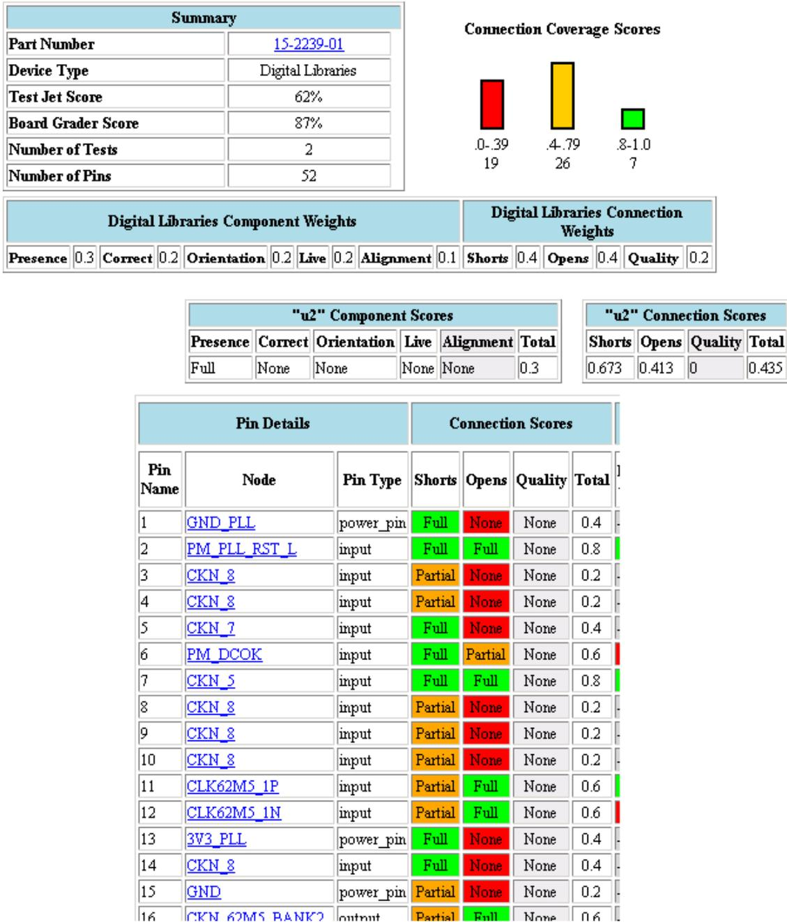
Figure 6: A portion of the coverage data for digital device "u2".
