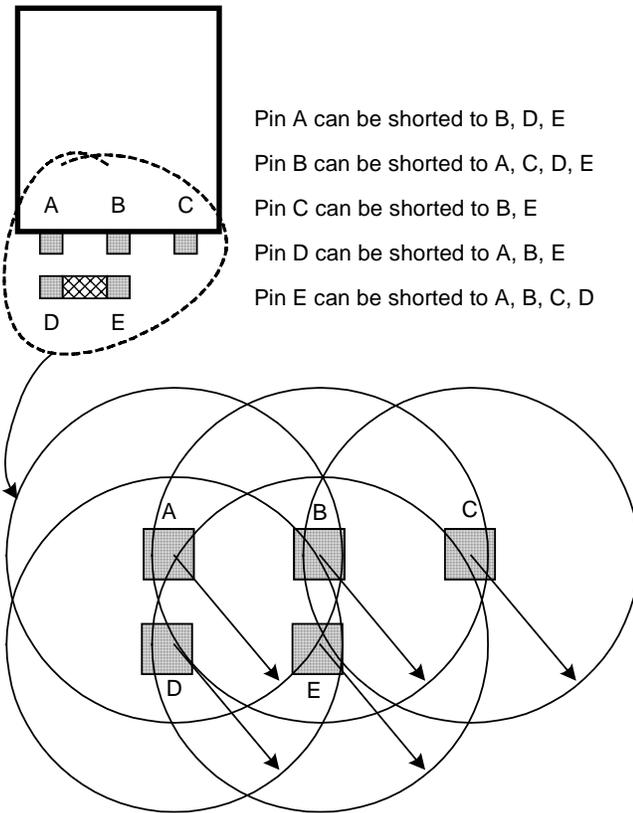
**Figure 1: Shorts are unwanted connectivity between connection points within a shorting radius.**
