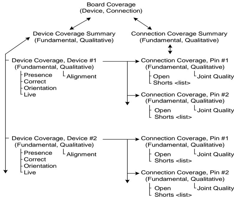
**Figure 2: Device and connection coverages summarized and detailed.**
