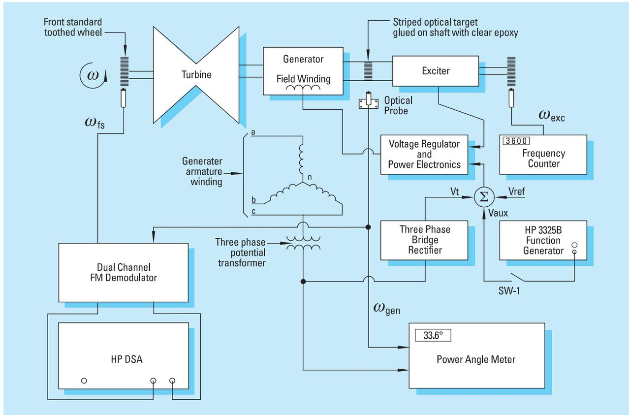
5 degrees offered by the old strobe and chalk line approach. DSAs deliver much more information, too, including key parameters such as overshoot and settling time. And the DSA is much safer, since test personnel don't need to be near an operational machine in order to make measurements. Figure 2 shows a typical instrumentation setup for measuring power angle.
