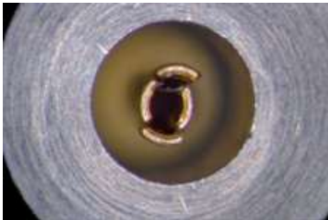
Damaged female centre conductor fingers on a 1.85 mm connector (photo courtesy of Jürg Rüfenacht, METAS, Switzerland).
