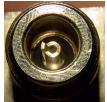
A bent female centre conductor finger on an N-type connector (photo courtesy of Tuomas Haitto, Finnish Defence Forces)
