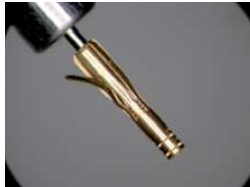
A bent 3.5 mm female centre conductor finger. The centre conductor has been removed here for replacement (photo courtesy of Jürg Rüfenacht, METAS, Switzerland).
