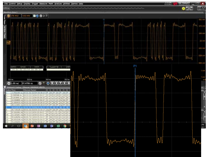
Figure 4. The 64b/66b includes a viewing pane and alignment marker, making it easy to identify problems in the system.
