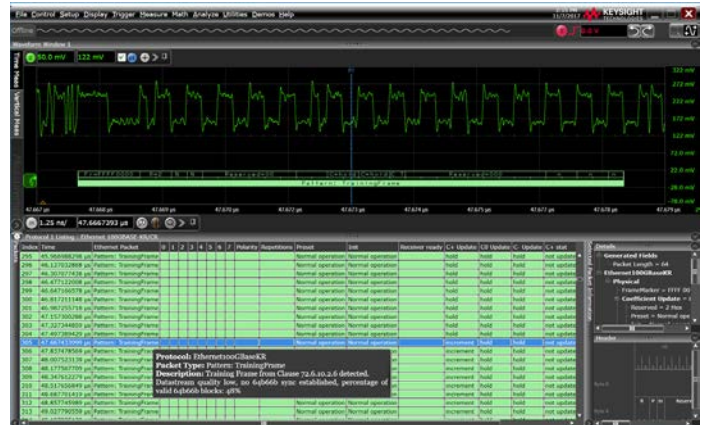
Figure 6. Training sequence of 100GBASE-KR/CR ethernet.
