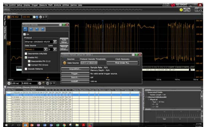
Figure 3. Customize your decoding setting using the manual tab. Image above shows the manual menu option.
